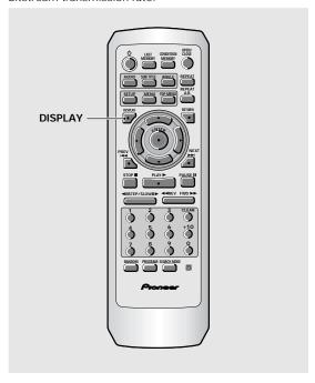
Press DISPLAY during while a disc is playing. Press DISPLAY repeatedly to change the information being displayed.
